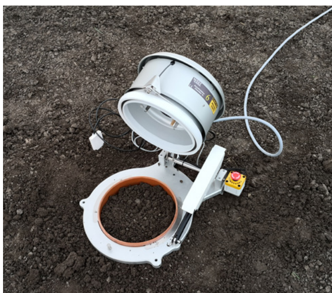
The prototype installed in the demonstration site (above) and detail of one of the chamber. The chambers close at fixed intervals to do the measurements of GHG fluxes from soil.
